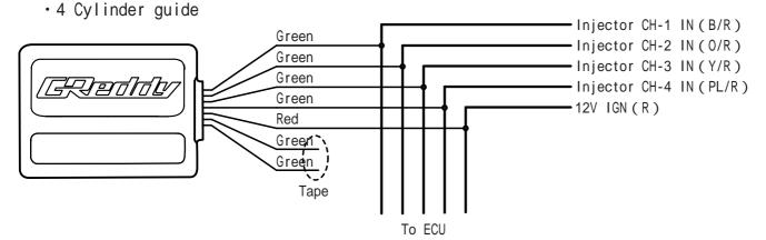
If green wires remain disconnected, please tape the ends to prevent short circuit.
