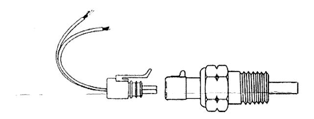
**Housing Material:** Brass with 3/8" NPT Thread (Torque to 25 Ft-Lbs) **Elec. Termination:** Integral weatherproof connector, Includes mating connector with 6" leads, 18 AWG. Black (Ground), White (Output)
