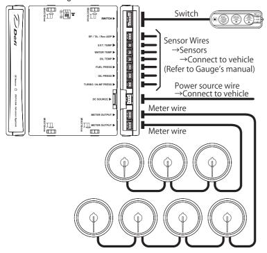
The meter wire can be connected to both two connecters of METER OUTPUT. Up to 7 gauges can be connected to each unit. (ex. If 7 gauges are connected to one line, none is connected to the other line.)
