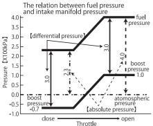
About differential pressure display of fuel pressure; Generally, fuel pressure of electric controlled engine car is controlled to keep in same ratio to intake manifold pressure by fuel pressure regulator. As shown in the graph, fuel pressure meter displaying absolute pressure value indicates 400kPa when boost pressure is 100kPa in case that differential pressure is set at 300kPa. Fuel pressure meter displaying the differential pressure value indicates 300kPa.
